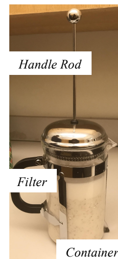
Figure 8: Almond Press Prototype detached with Rod to contain nylon mesh filter
